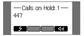
Pressing the flash key again will resume the call. While a call is on hold, you can establish another call by dialing the desired number. When more than one call is on hold the following window appears.
